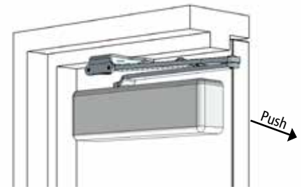
Parallel Arm (Push Side) Permits 180° maximum opening
